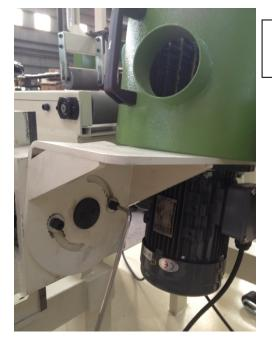
The Left and Right sanding head can adjust to Tilt
