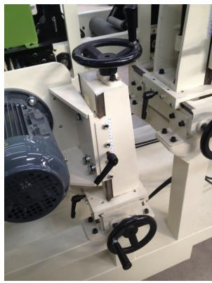
The separated position of the upper sanding head and lower sanding head.
