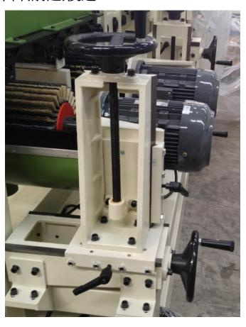
2. The Right & Left side of the sanding head can to adjust separately upward,down ,forward and backward
